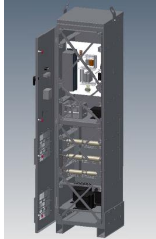
3D Model of an HRG assembly indicating bracing and reinforced mounting feet.
